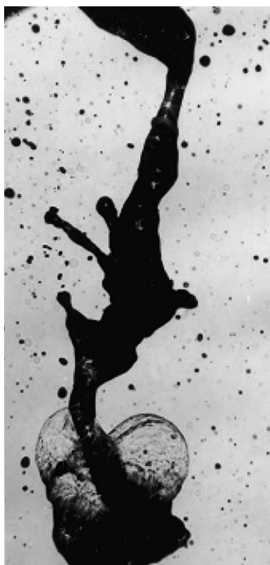
Figure 13. Membrane-fiber breakup of high-speed round liquid jet in still gas. ( We = 38 ) 30
